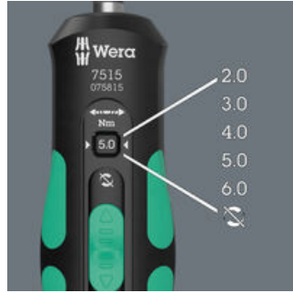
Five selectable tightening torques (2.0; 3.0; 4.0; 5.0; 6.0 Nm) and one fixed position (Torque Lock) for unlimited tightening and loosening moments.
