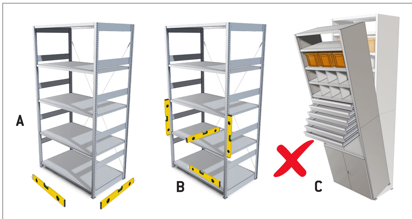
Figura 14 Support floor, levelling and fixing
